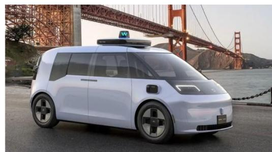
equipped with 13 cameras, four lidar units, six radar sensors, and external audio receivers. It is intended to be a mass-produced vehicle made to Waymo's specifications. At present it is undergoing tests in the United States. More information and a short video are at [this link](#).
